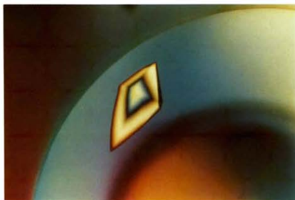
Fig. 1. Tetragonal crystal of glutathione peroxidase from human plasma. Space group I4_1 , a = b = 83.1 and c = 131.0 Å. The maximal dimension of the crystal is about 0.5 mm.
